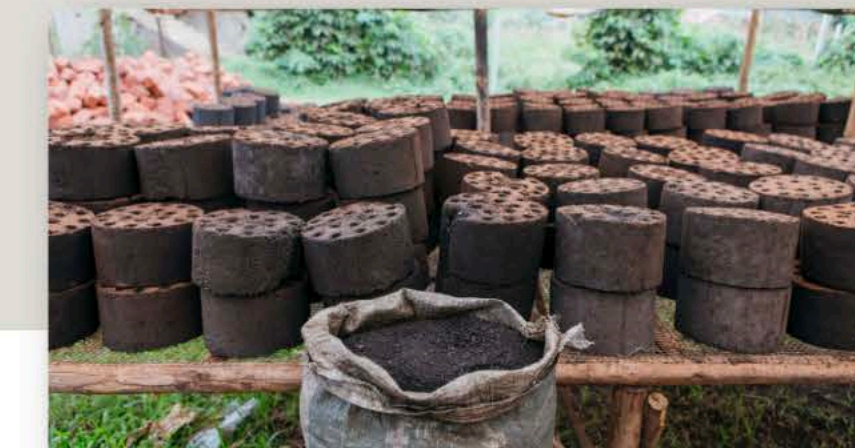
Making fecal sludge cooking briquettes for cookstoves (honeycomb shaped) and stick (for clay ovens)
