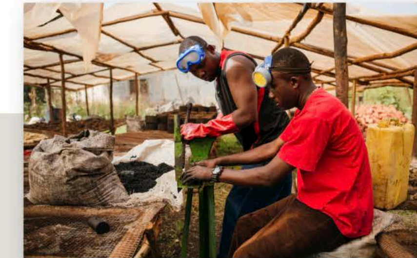
Making fecal sludge cooking briquettes for cookstoves (honeycomb shaped) and stick (for clay ovens)
